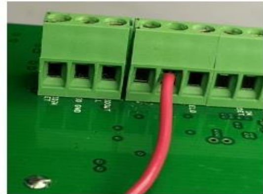
GOOD, WIRE "IN" THE SCREW CLAMP NOT UNDERNEATH
